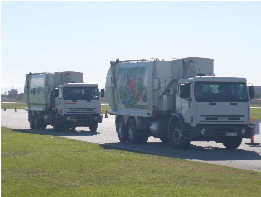
Drive Evaluation SIBS Truck Underway on Test Track
